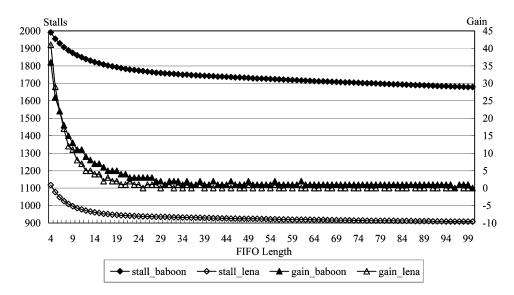
Fig. 15. Influence of the FIFO length on number of stalled cycles. Gain means the number of stalled cycles decreased by the increase of the FIFO length.
