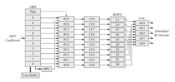
Fig. 5. Block diagram of the proposed architecture. Only the MPC module involves word-level computations, and all other modules process independently over bit planes.
