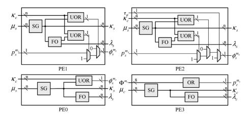
Fig. 8. Circuit of the PEs in the MPC module. The  $\kappa_s$  and  $\lambda_s$  are passed to next stage. The  $\phi_s^{m_c}$  of the PE0–PE2 is used by the PE3 to generate the main output,  $P_c^{m_c}$ , of the MPC module.
