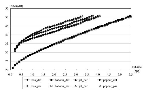
Fig. 4. Comparisons of rate-distortion curves of various images of parallel mode and default mode. All the images are of size  $512 \times 512$  coded by 5/3 filter with two levels of decompositions,  $128 \times 128$  tile and  $64 \times 64$  code block.
