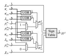
Fig. 11. Circuit for computing the  $H^{\chi}$  of sign coding. It can be used to compute  $V^{\chi}$  by replacing the corresponding inputs.
