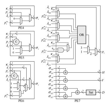
Fig. 10. Circuit of the PEs in the PC module. The superscript, k, indicating bit plane number is omitted for simplicity.
