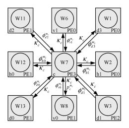
Fig. 7. Interconnections between the PEs in the MPC module. The PE3 classifies the coding pass of the MSB of C,  $p_c^{m_c}$ , into one of the three coding passes, and merges  $p_c^{m_c}$  into the dataflow of the GRB module.
